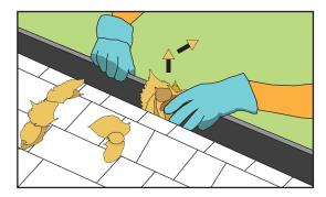
Try to keep gutter guard at the same pitch angle as the roof
